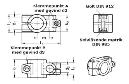
Adjustable clamp lever for d3 = GN 911-M10-55 have to be ordred separately 11 = 122.0Adjustable clamp lever for d4 = GN 911-M 8-32 have to be ordred separately 12 = 65d1 13 = 40= 48= 20 m = 45d2 = M10d3 = M 8d4 = 65 k1
